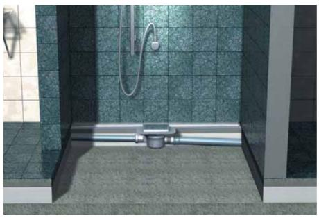
The *Linearis* shower channel features a narrow, elegant stainless steel channel ① which can be discreetly integrated into the bathroom design. With a flow capacity of 24 liters per minute the *Linearis* shower channel is ideal for mounting against the wall at the back of the shower. For cleaning and maintenance purposes the stainless steel channel and tileable access opening ② can be removed allowing full access to the odor trap and drain body.
