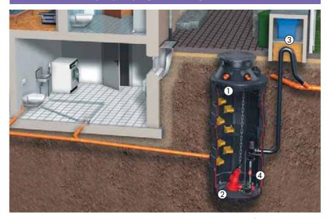
Domestic wastewater flows with natural gradient to the pumping station ① and is pumped by the integrated TPF macerator pump ② over long distances (pressure draining) into the sewer. The pressure pipe ③ should always be laid frost-free. A control unit takes over the fully automatic pump control from within the building. Float switches ④ are used as level sensors. The system complies with the ATEX product directive and is suitable for installation in potentially explosive atmospheres.
